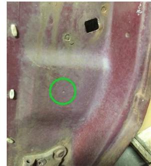
Like the door, the door jam/cowl might already have a small hole drilled. Drill a 1 7/8" hole on center with this hole for the conduit.
