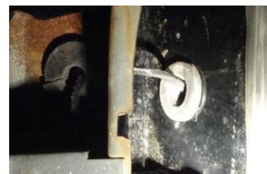
The power window regulator only shares one hole with the manual regulator. This picture shows the approximate orientation of the new regulator when it is installed in the door.
